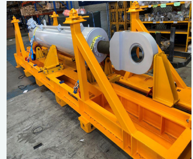
Image 1: Hydraulic Boom Luffing Cylinder
